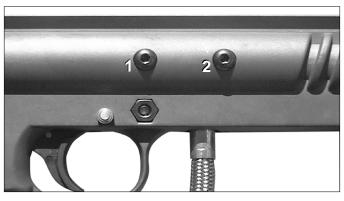
To release the power tube and valve, unscrew the two valve bolts on the outer right-side receiver.
